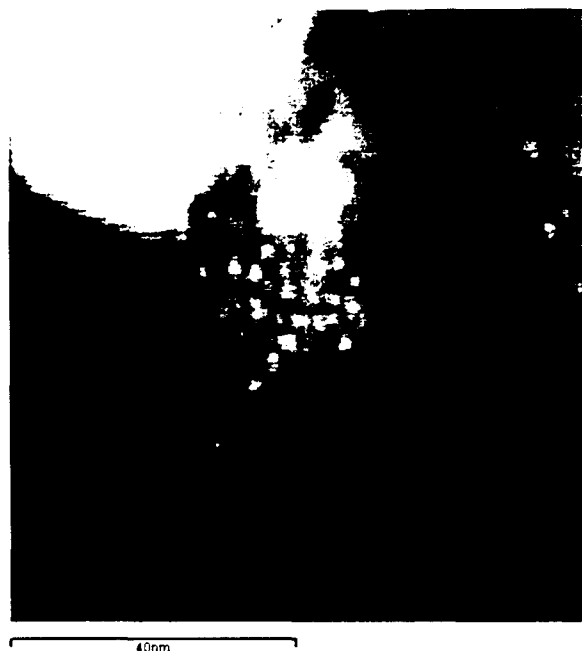
Figure 24 - HAADF image of small Au particles in sample Z2, [1 MX]
