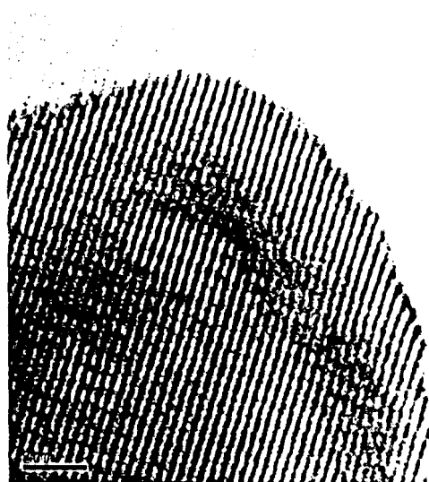
Figure 22 - HRTEM lattice image of ZnO catalyt showing [110] plane spacings (0.17 nm) [3 MX]
