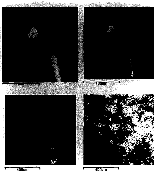
Figure 37 - HAADF image (top left) of 2.5%Au-2.5%Pd/TiO 2 sample and corresponding XEDS maps of Au (top right), Pd (bottom left), and Ti (bottom right), [100 kX]
