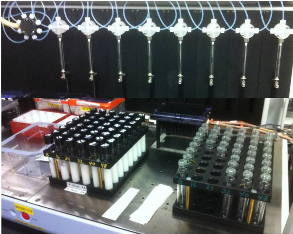
Picture A 2. Janus Formulator Components; Dispense Pumps (top) and Sample Tubes (bottom)
