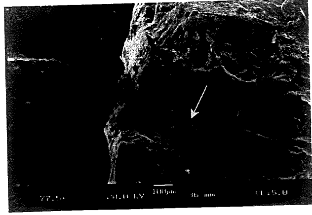
(c) View of Hole due to Slag Inclusion
