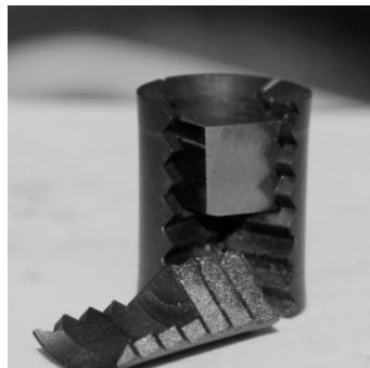
Figure 8. a) Fragment Simulating Projectiles (mm scale), b) 4 Piece Sabot Shown with Cube FSP
