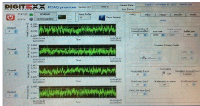
Figure 7.5. PDAQ data acquisition from Silicon Design 2210 accelerometer
