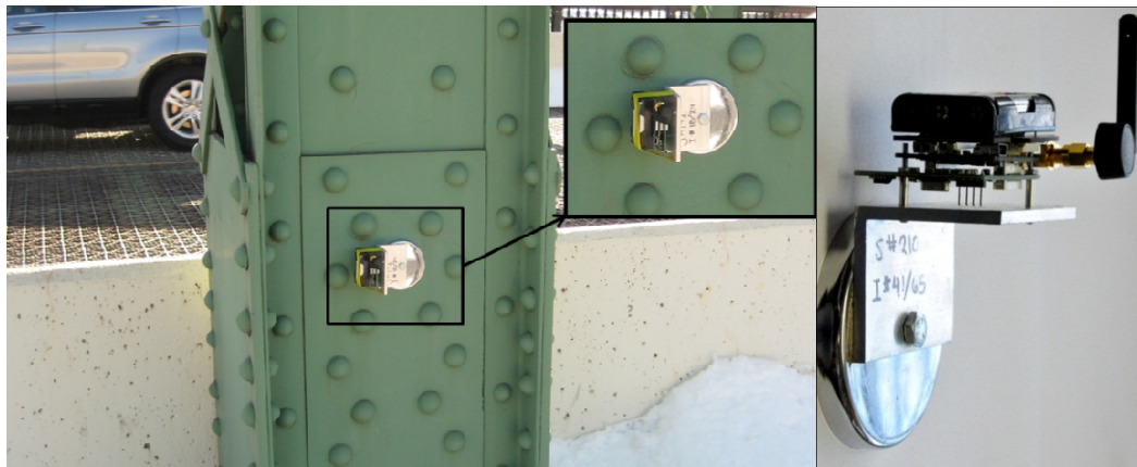
Figure 7.3. Sensor attachment using magnet connections
