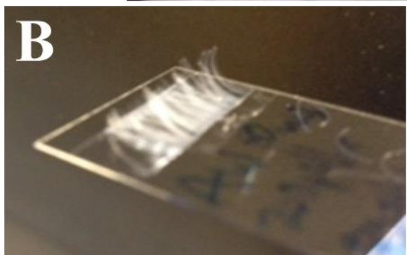
Figure 5.8: Photographs of delaminated thick nanoparticle cracks. (A) In-situ photography of experimental setup highlighting substrate and blade. (B) Substrate after coating completion. Note the delaminated, “peeling,” cracks (C) Deposition blade. Some delaminated nanoparticle cracks wetted and adhered to the deposition blade.
