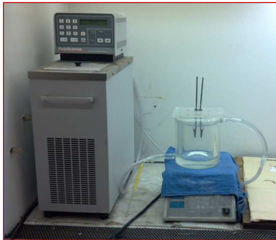
Figure 7. Recirculating chiller and double-walled beaker used as the anodization chamber in this experiment
