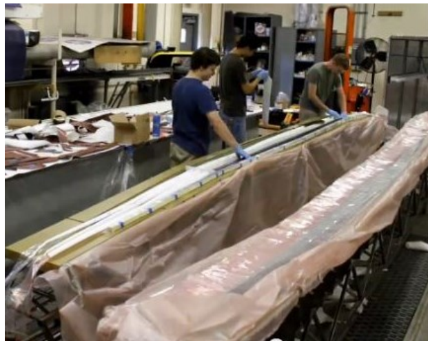
Figure 46: Laying Web Plies over Foam Molds
