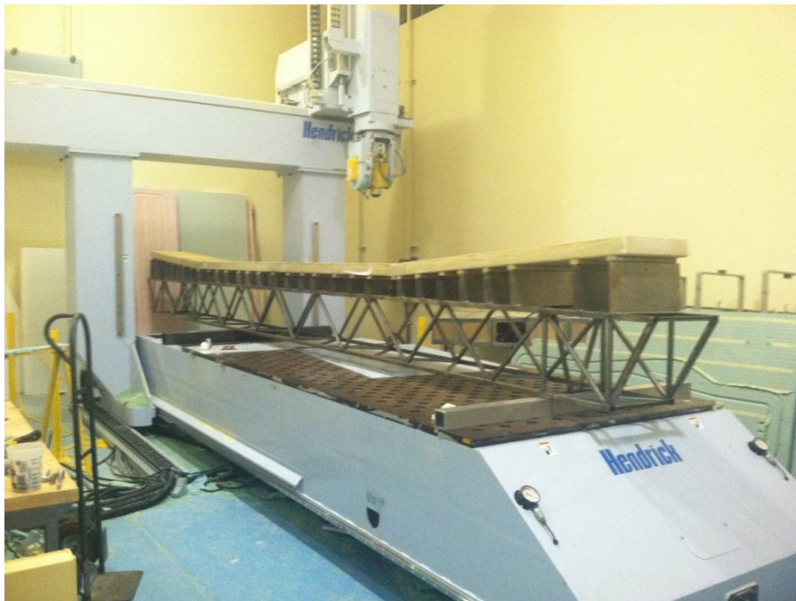
Figure 38: Mold Setup for Machining
