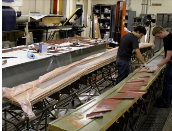
Figure 44: Debulking First Ply and Continuing Layup
