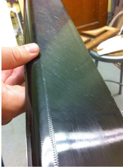
Figure 61: Typical Control Surface Finish
