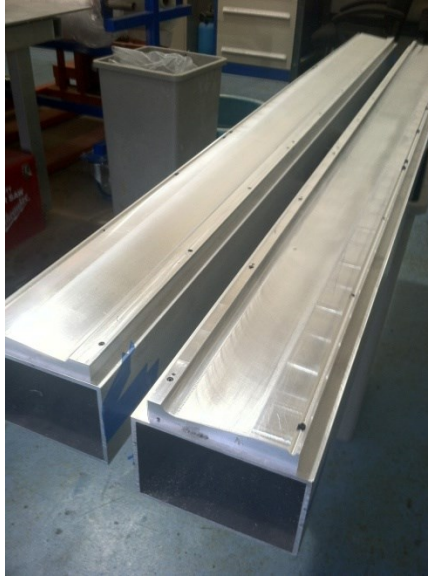
Figure 60: Finished Flap Molds
