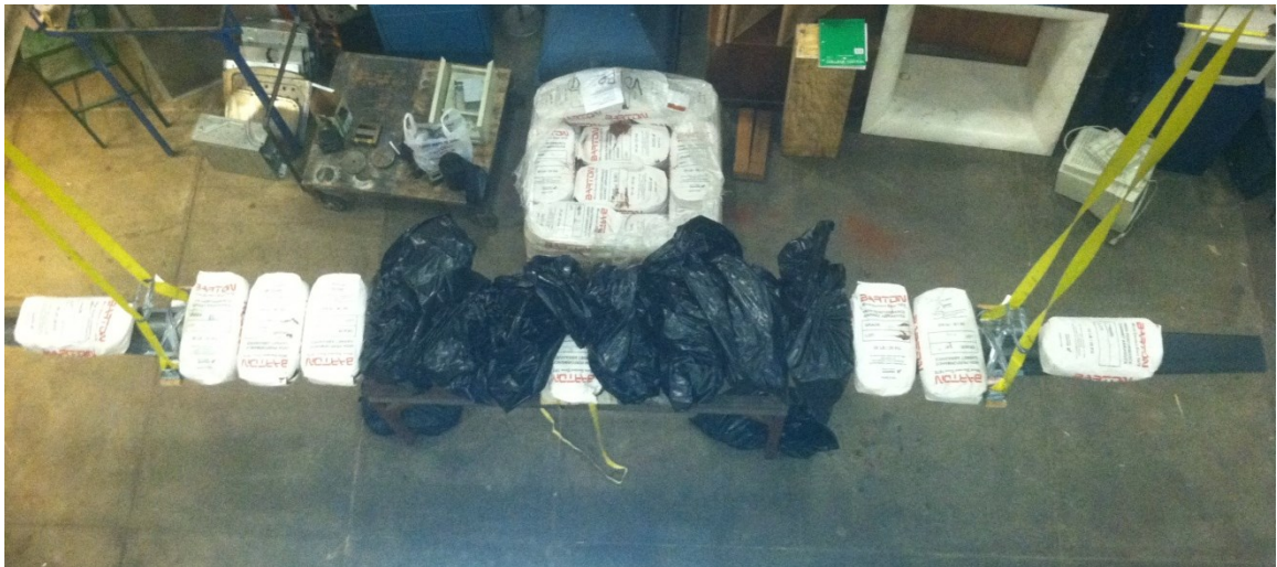
Figure 50: 3.5 KN Proof Load of Wing
