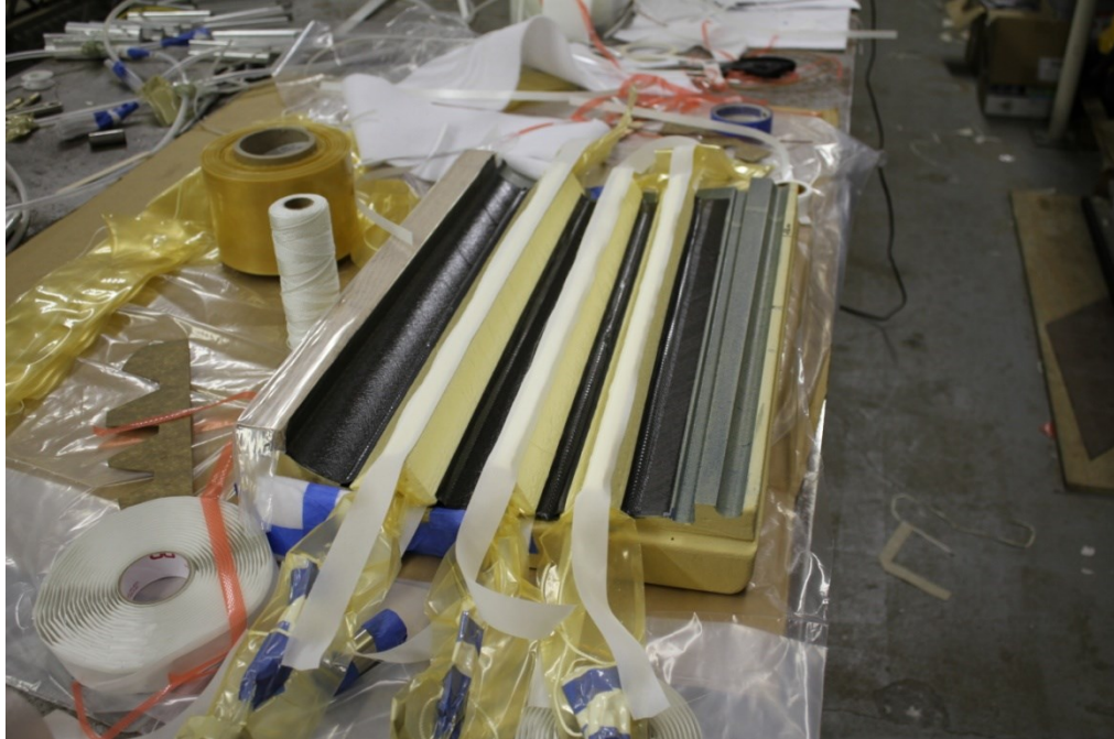
Figure 24: Placement of Foam Molds
