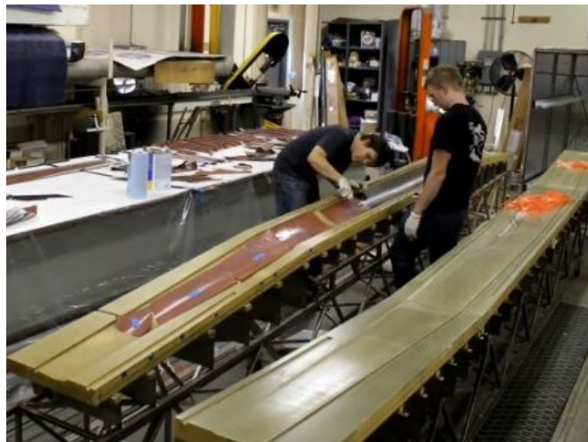
Figure 43: Laying of 1st Wing Skin Ply
