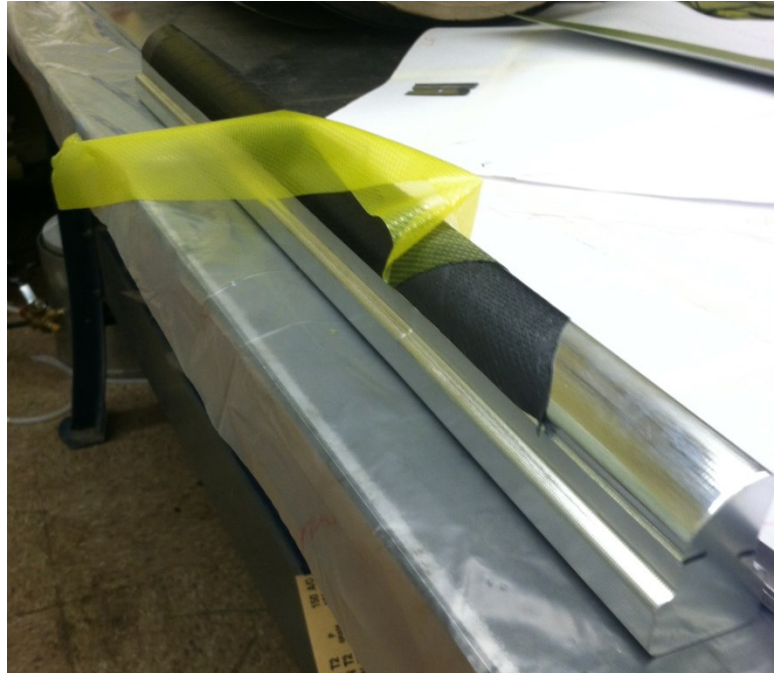
Figure 17: Trailing Edge Layup
