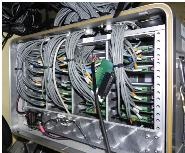
Figure 4-7: Compact DAQ Instrumentation
