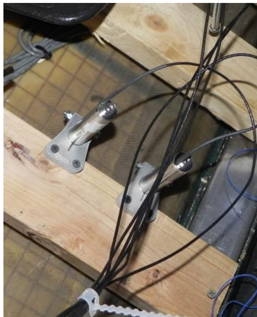
Figure 4-9: LVDTs mounted for static load tests
