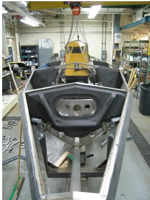
Figure 3-14: Assembly of bulkhead panels and side panels
