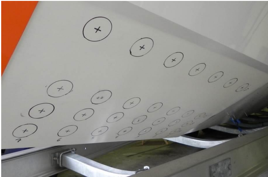
Figure 4-10: Static load test grid
