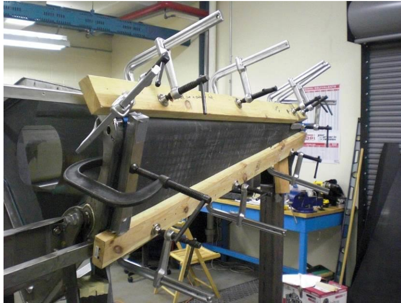
Figure 3-15: Bonding of a side panel
