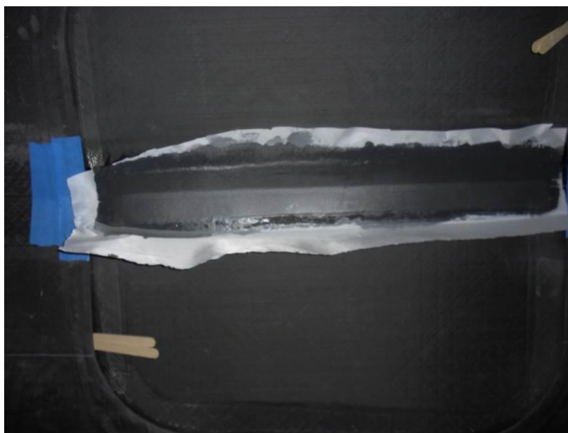
Figure 3-17: Reinforcement fiber cloth wet laminated to a panel.
