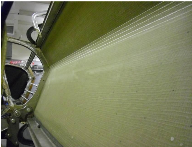
Figure 3-16: Scores on the inner side of a bonded side panel.
