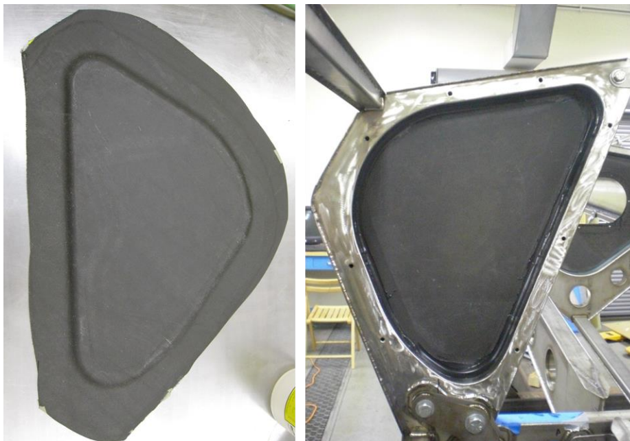
Figure 3-12: Demolded composite bulkhead panel and the bonded panel
