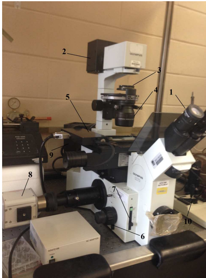
Fig. 14 Olympus IX70 acts as measurement equipment
