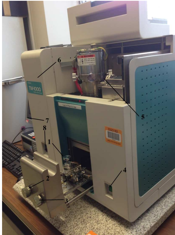
Fig. 15 Hitachi Tabletop Microscope acts as cross-section observation equipment
