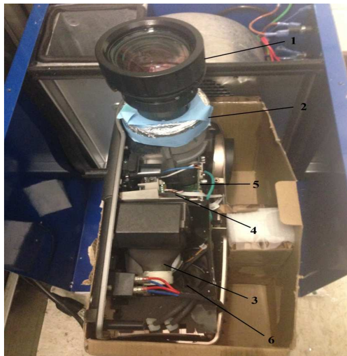
Fig. 13 Inside of Microlithography device with addition distance from lens to DMD
