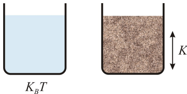
Figure 1.1: (left) Equilibrium thermal system – ink drop in water after a long time and (right) non-equilibrium athermal system – vertically vibrated sand filled beaker .
