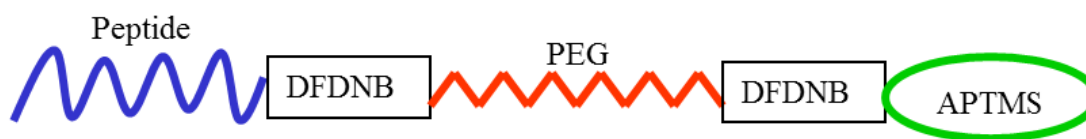
Figure 4.4. Schematic of assembled PEG-peptide complex. DFDNB is used as a crosslinker to link the peptide to PEG and PEG to a silane to allow for further binding with the silica NPs. (not to scale)
