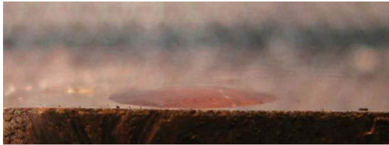
Figure 3.5 A droplet of a fluorinert (3m Novec Fluid HFE-72DE) is placed on a polished copper surface that has been prepared with a fluorinate self assembled monolayer. The contact angle is less than 10^\circ .
