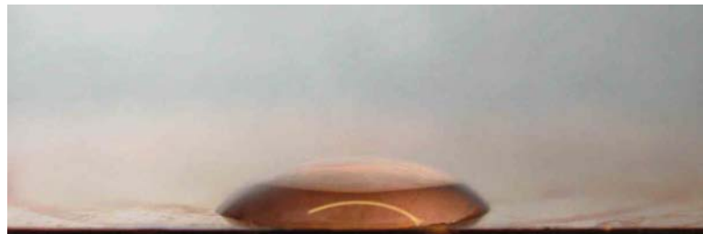
Figure 3.6 A droplet of methanol is placed on a polished copper surface that has been prepared with a fluorinate self-assembled monolayer. The contact angle is roughly 40^\circ .
