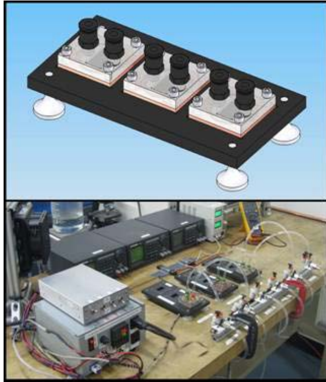
Figure 6.4 Illustration corrosion and erosion test apparatus.
