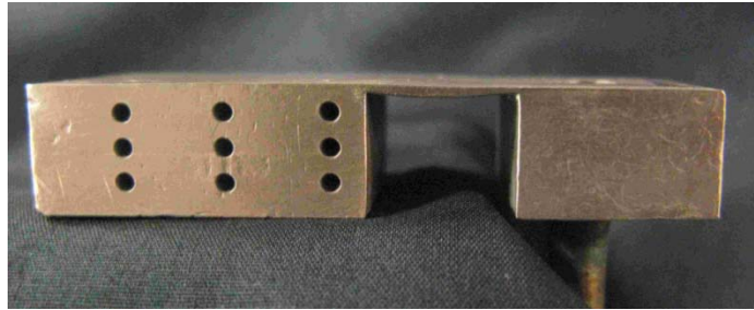
Figure 2.5 Shows a side view of the test section. Thermocouples inserted in the 9 holes are used to measure the heat flux and surface temperature of the condensing surface. A gap was also machined to prevent heat from leaking in through the vapor/liquid ports.
