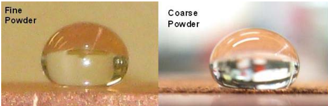
Figure 3.4 Photograph of water droplet on one layer of powder after treatment of the surface with a self-assembled monolayer of hydrophobic octadecyl mercaptan.
