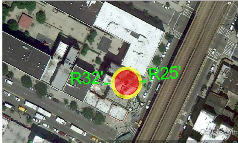
Figure 48 Growing area of buildings damage for Harlem accident (Pso =5.0 psi)
