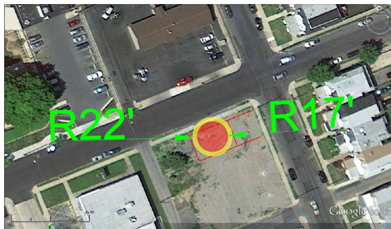
Figure 46 Growing area of buildings damage for Allentown accident (Pso =5 psi)
