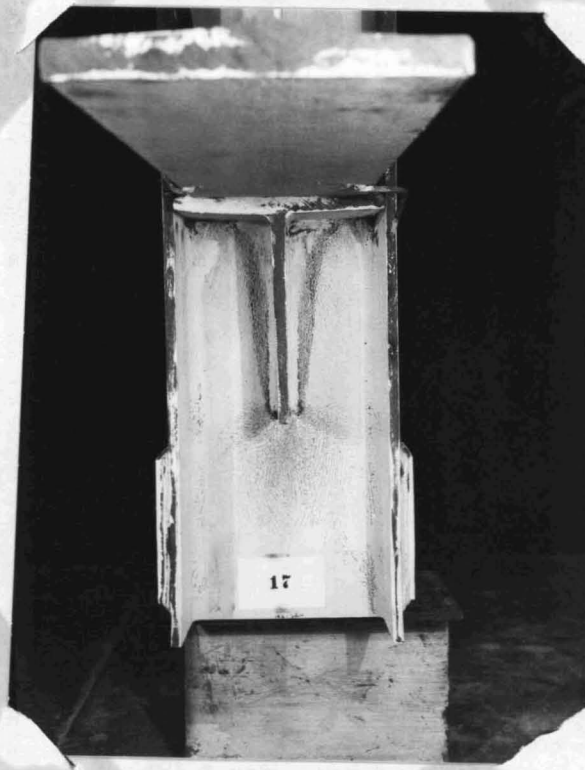
Fig. 52(b) - Strain Pattern In Column Web Around Tee
