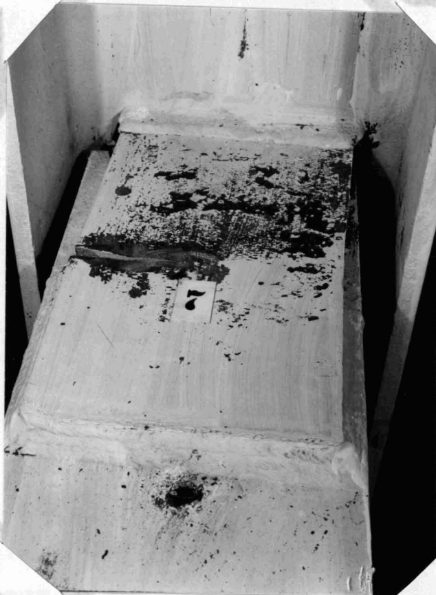
Fig. 20(b) - Top Plate Failure of Test 7
