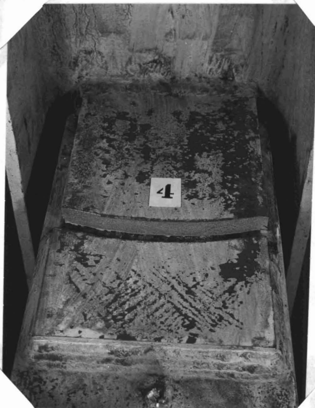
Fig. 17(b) - Fracture of Test 4 Top Plate
