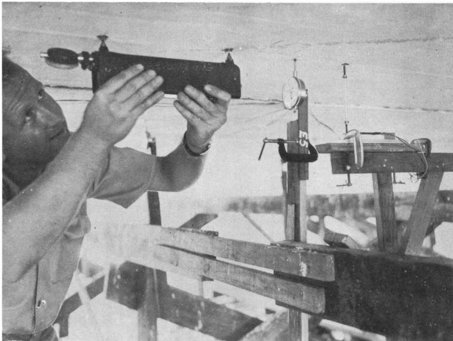
Fig. 7 Detail of the Installation from Left to Right (a) Whittemore gage for strain measurements (b) Ames gage for the deflection (c) Dynamic gage
