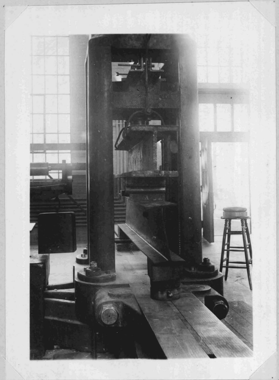
Fig. 2 - End View of Beam No.2, Bethlehem B12-28 Section Showing Failure Due to End Twisting
