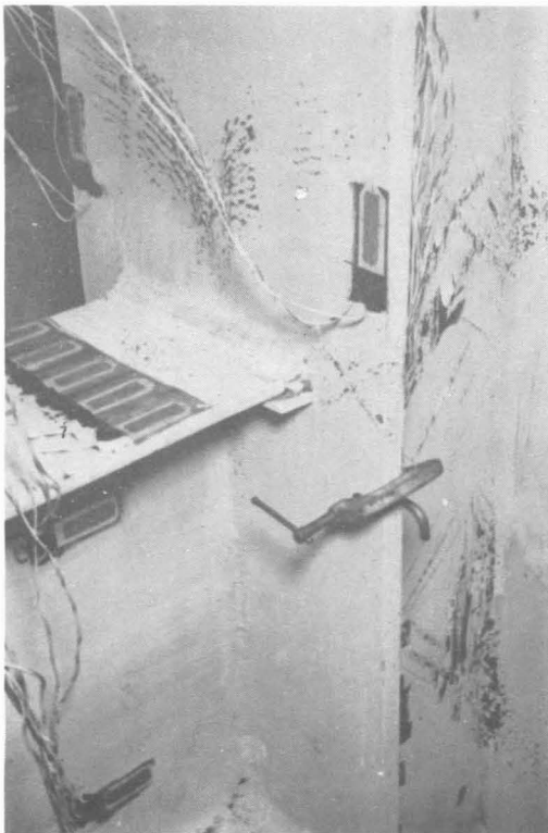
A-4 At Maximum Load of 44 Kips on Each Beam
