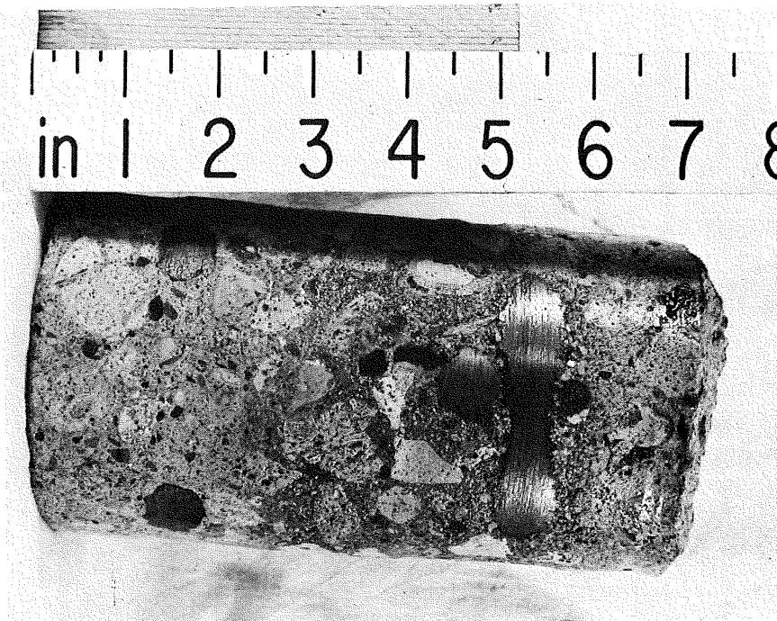
Fig. H-34 Cores Taken From Impregnated Area of Bethlehem Spur Route Bridge Deck; Photographs Taken After Etching with 15% HCl
