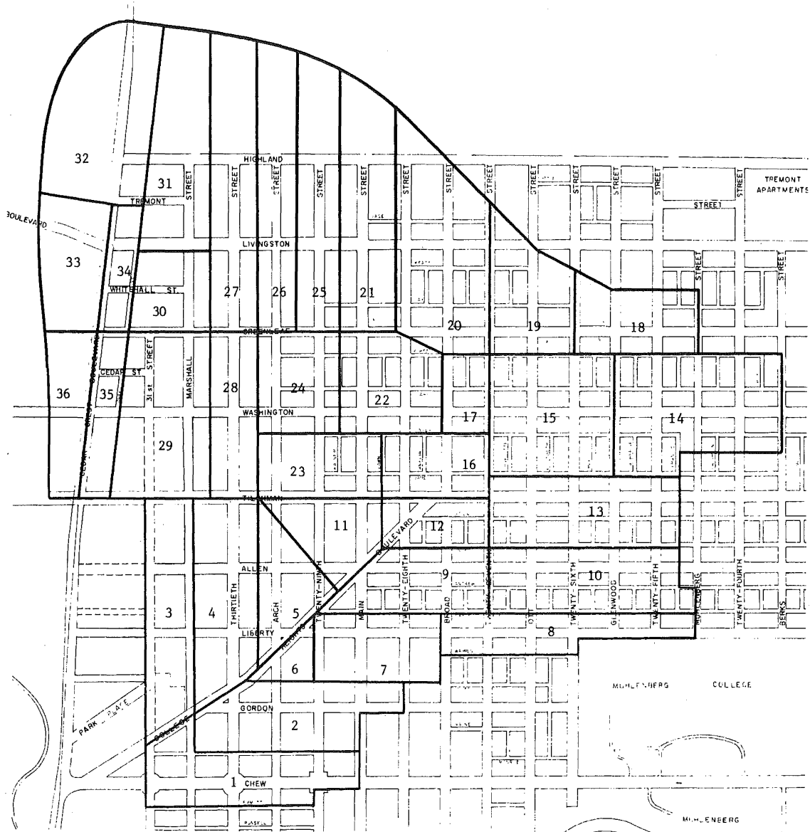
Fig. 3 COLLEGE HEIGHTS BOULEVARD DRAINAGE SYSTEM SUBCATCHMENTS
