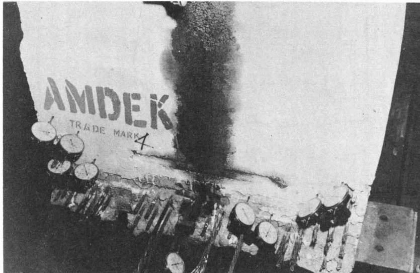
Fig. 5 - End View of Beam Showing the Dials for Measuring Slip of Strand at Release of Prestress
