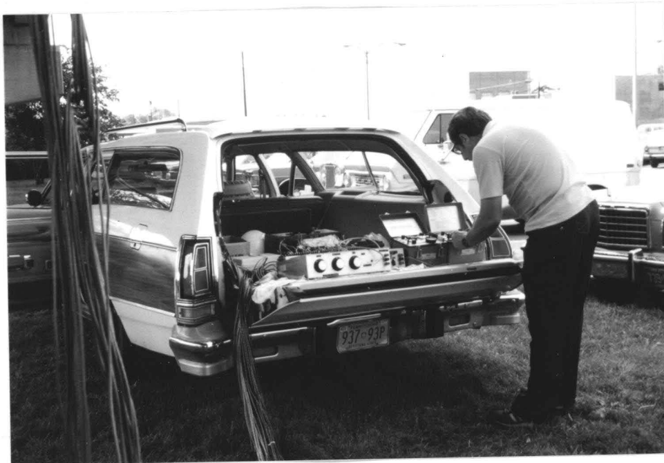
Fig. 9 View of Switch Box, the Two Indicators and the Two Cables leading to the Terminal Boxes on the Safety Rail and on Top of Pier
