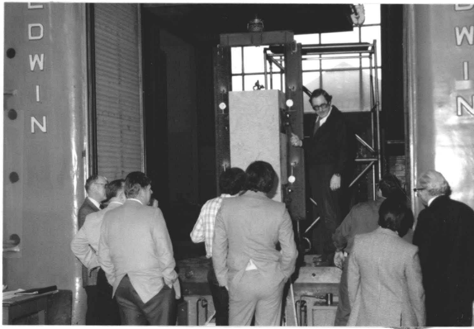
Fig. 18 Compression Rail Anchor Restraint Test in Progress
