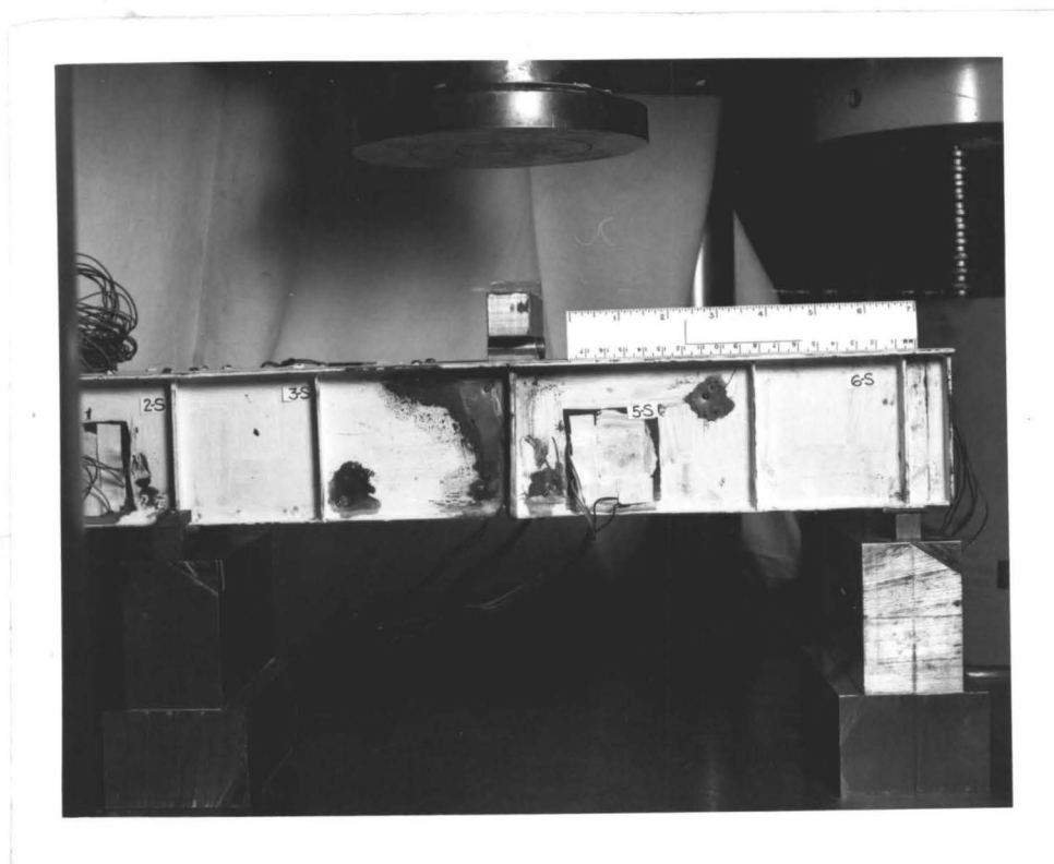
Fig. 2.16 TEST SETUP FOR SPECIMEN M2 (Symmetrical Loading)
