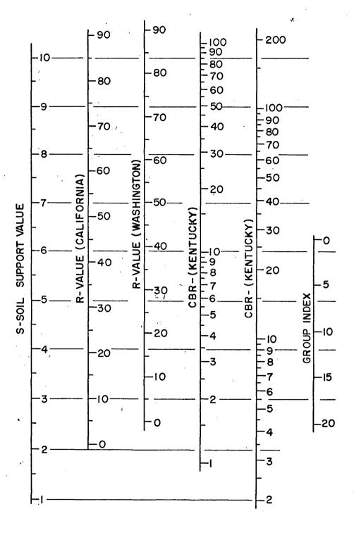
Fig. 3 AASHO Correlation Scale for Soil Support Values
