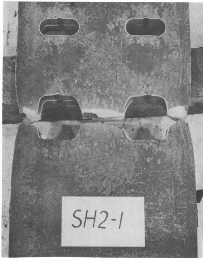
FIG. 19 Deformation of Slotted Holes
