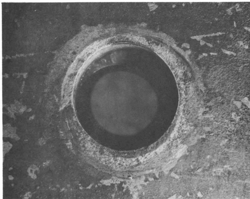
FIG. 11 Plate Area Under Turned Element Where a Washer Was Used - Joint OH3-2 (1/4-in. Clearance)
