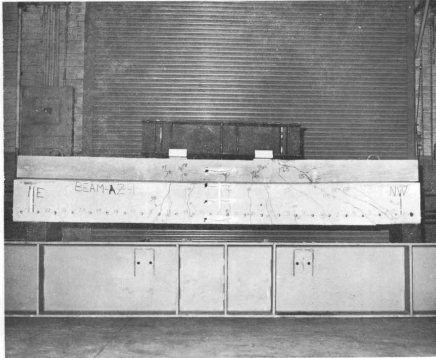
Fig. 9 Crack Pattern Beam Z-1
