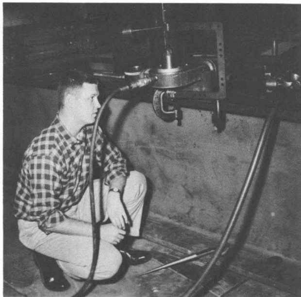
Fig. 4 C-Frame Extensometer in Place, Torqued Calibration
