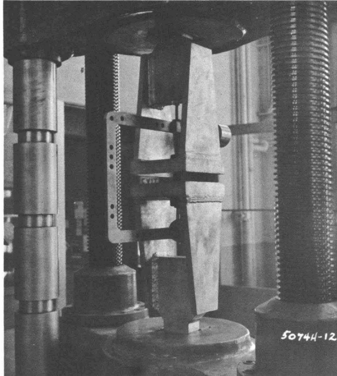
Fig. 7 Direct Tension Calibration
