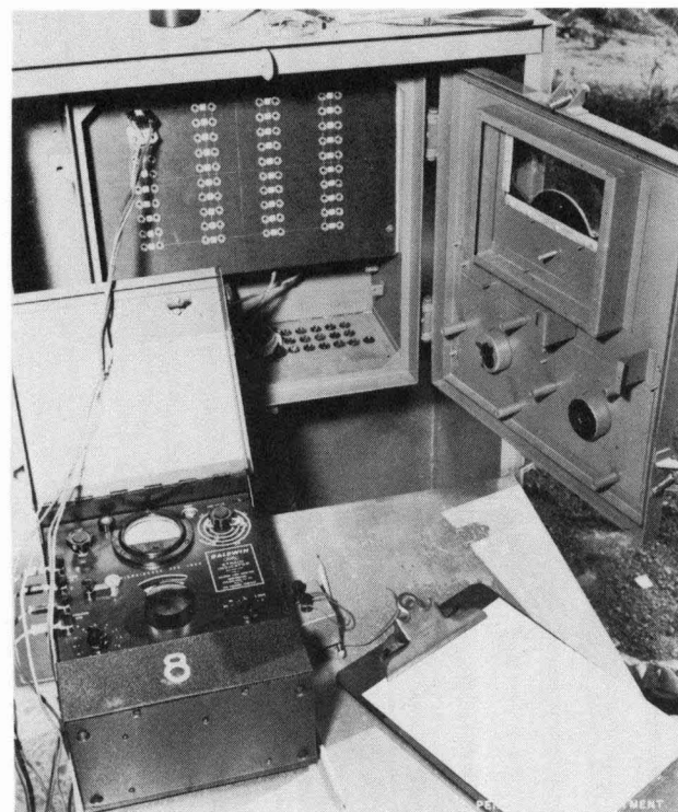
Figure 13 Terminal Board Ready for Gage Reading, Showing Indicator Box and Jack Plugs Inserted into Board
