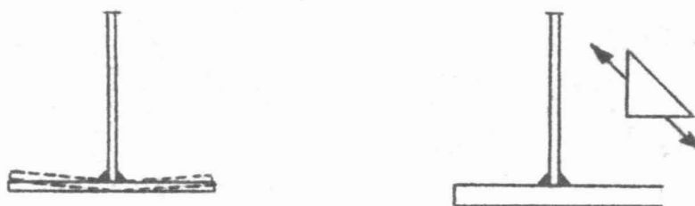
Fig. 2 Web-Flange Connection (Transverse Residual Stresses)
