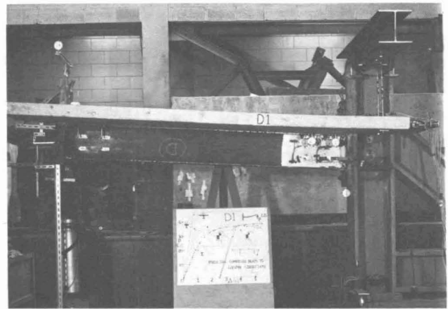
Fig. 20. Testing of composite beam-to-column connection
