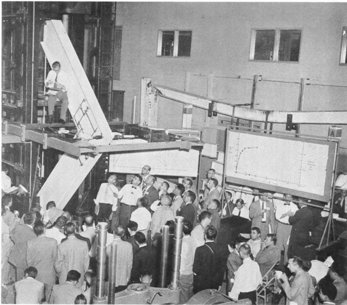
Test of a corner connection joining 30WF108 beam and column
