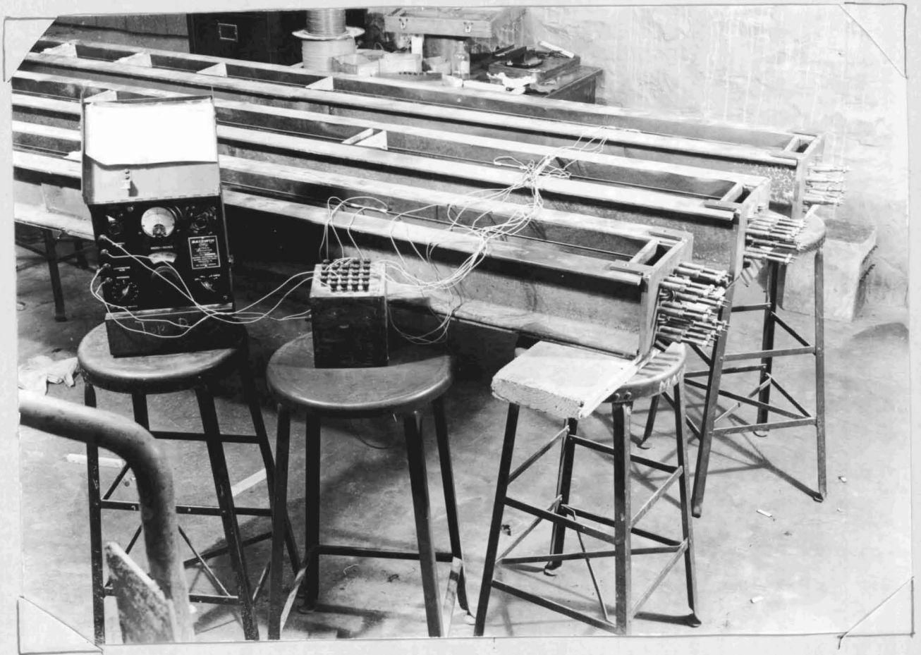
Figure (8) A-12, SR-4 Strain Gages On Wires For Checking On Prestress
