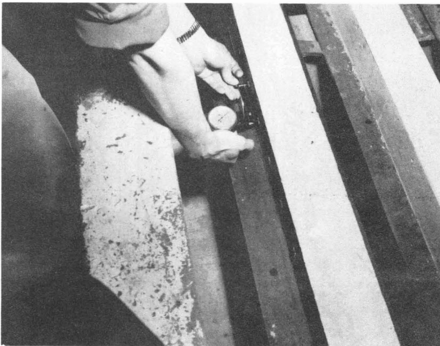
Figure 20 Huggenberger Ten- someter Measuring Concrete Strains
