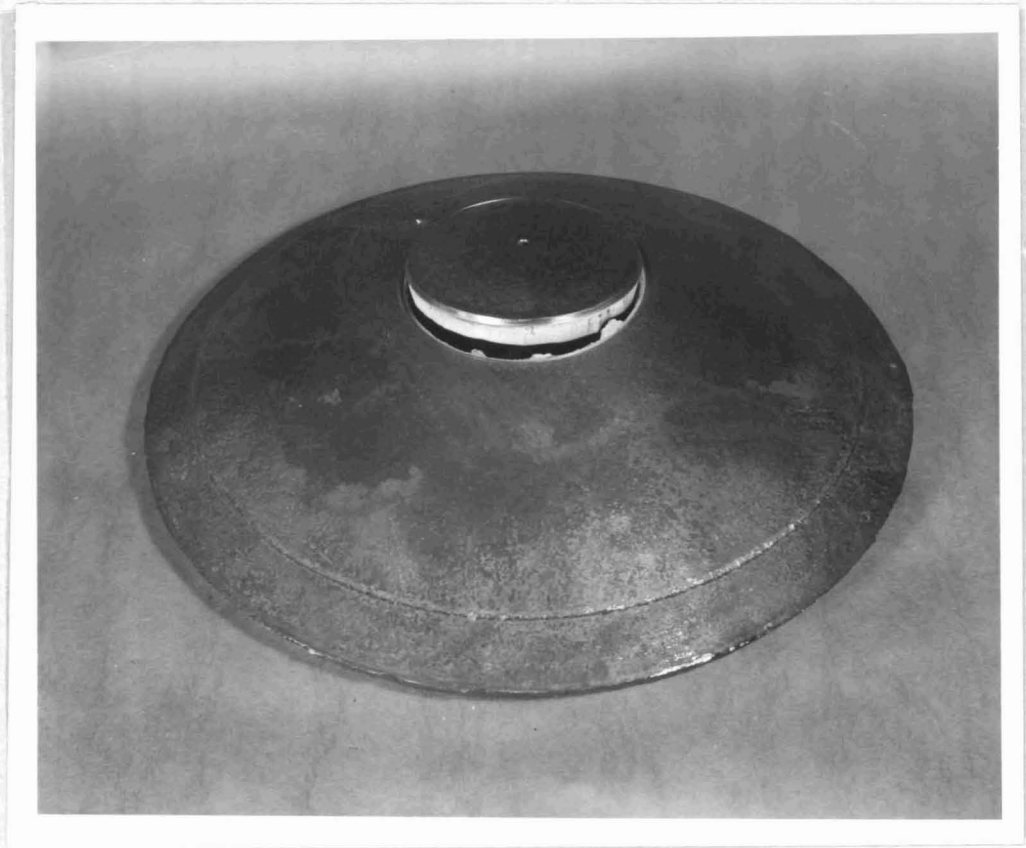
Fig. 35 SPHERICAL SPECIMENS Showing Typical Shear Fracture
