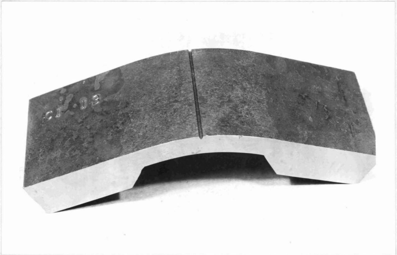
Fig. 2b Cylindrically Bent Specimen
