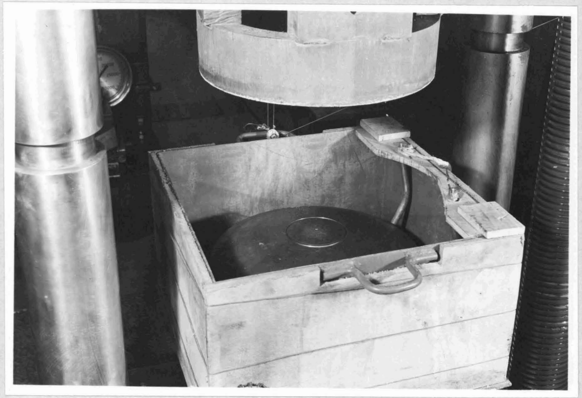
Fig. 6b. SPHERICAL TESTING SET-UP Showing Constant Temperature Bath with the Specimen Ready to be Tested.
