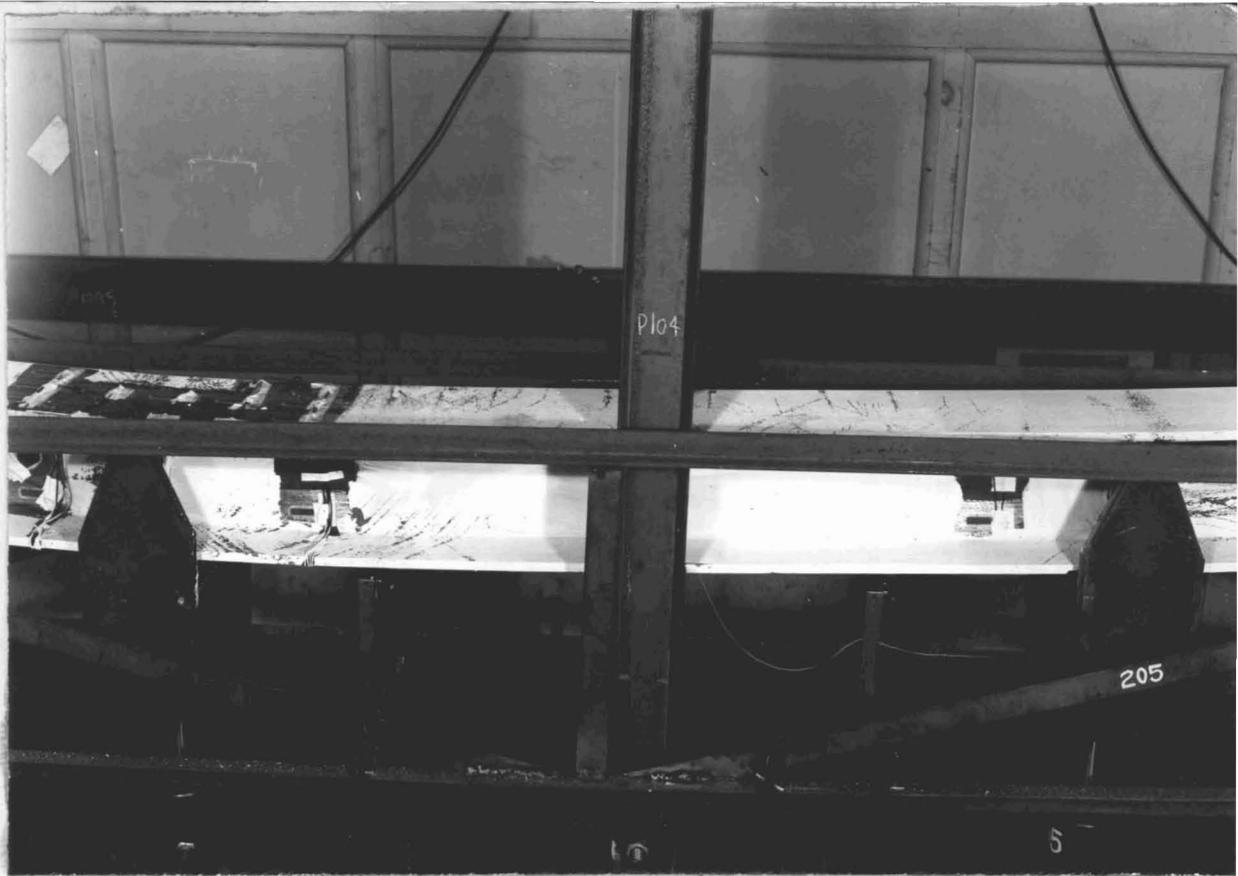
Fig. 28 . The progression of Lueder lines in the lower flange of the central span at a load  $W = 54$  kips in continuous beam test B2.
