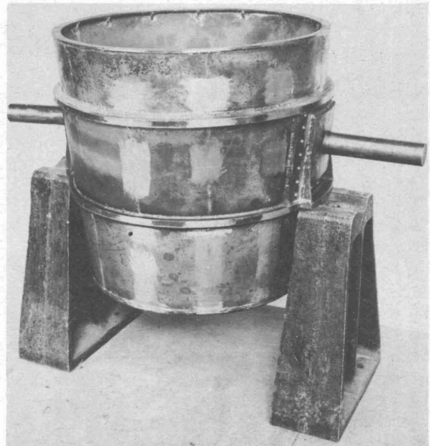
Fig. 1. Ladle Model. Height: 30 in. Top Diameter: 30 in. Surfacing for Outside Gages and Drilled Holes for Leads from inside Gages Shown.
