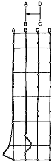
Fig. 10.—Carbon steel specimens loaded at kern point. Profiles of flanges of columns after failure.
