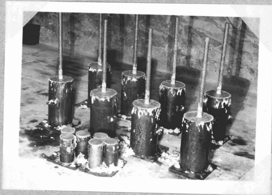
Fig. 3 - Pullout Specimens after Pouring
