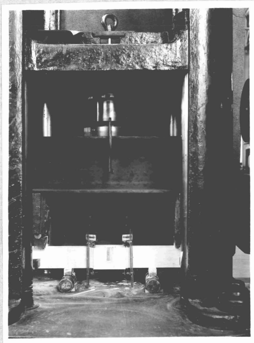
Fig. 6 - Specimen A 34 Set-Up In Pure Bending in 300,000-Lb. Machine
