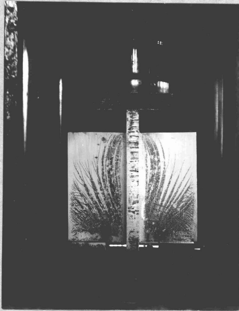
Fig. 15 - Specimen C 124 at Total Load of 240,000 lb.
