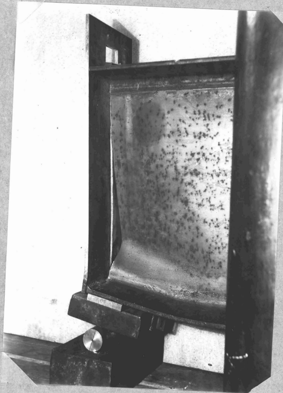
Fig. 6 - Beam CT-1, Showing Failure at the Support Due to Web Crippling
