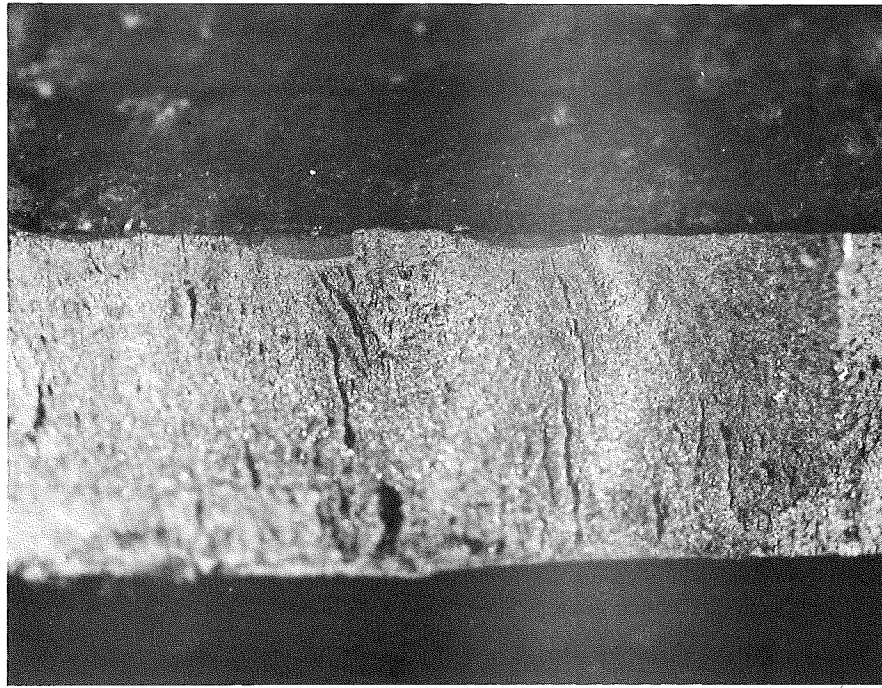
Fig. 31 Crack Development Along Transverse Weld Toe After 100 Million Cycles (Beam B1 - East Cover Plate)
