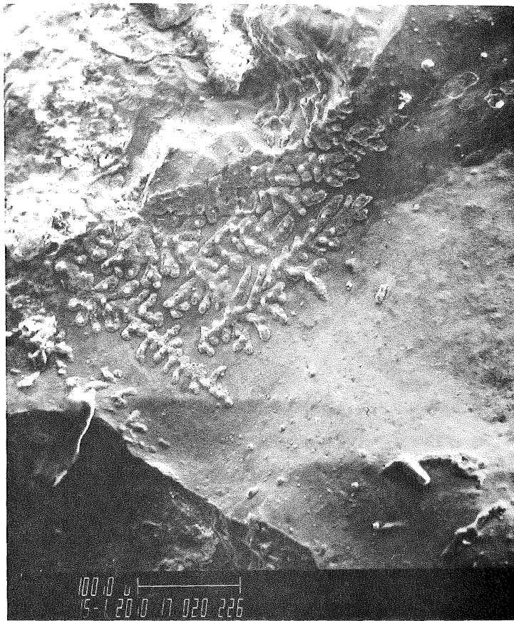
Fig. 58. SEM fractograph showing dendritic copper on the intergranular crack surface (Core F).
