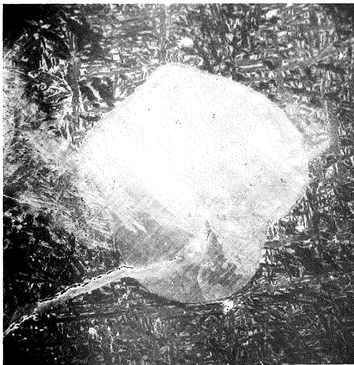
Fig. 53. SEM photograph of a crack emanating from a copper globule.
