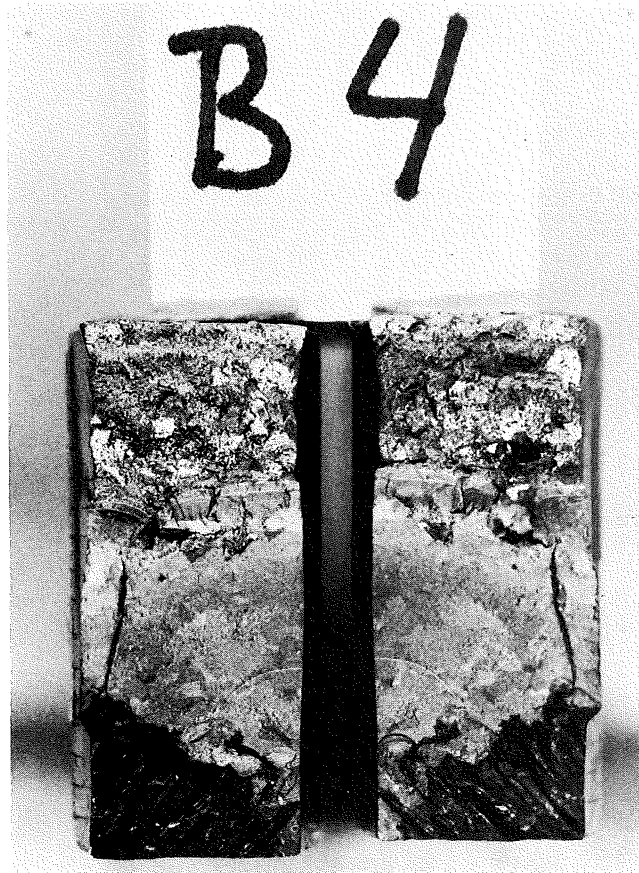
Fig. 33. Natural crack profile in specimen B4.
