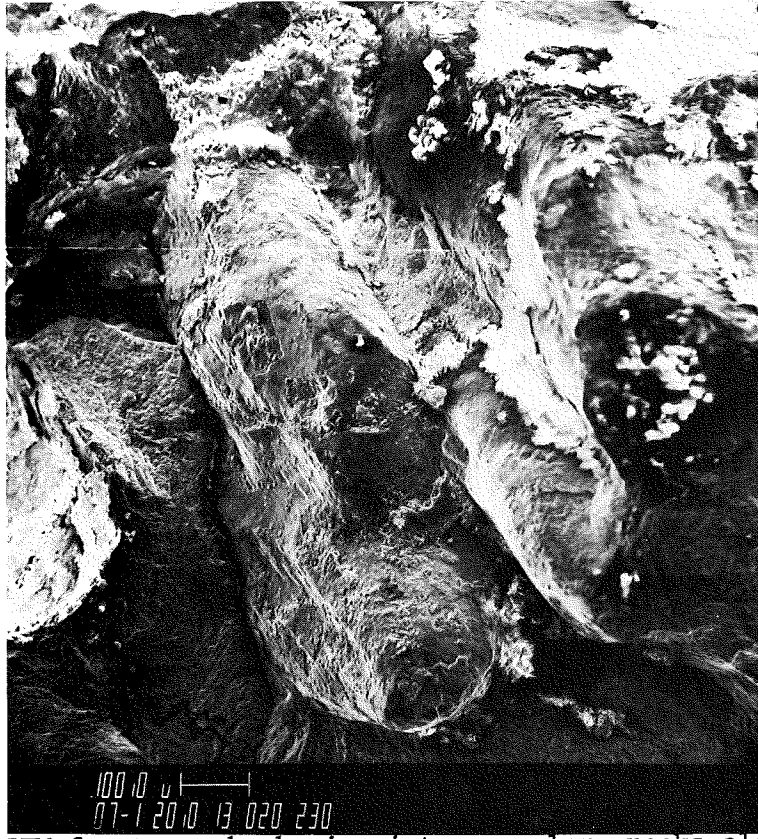
Fig. 56. SEM fractograph showing intergranular cracks along the large columnar grains.
