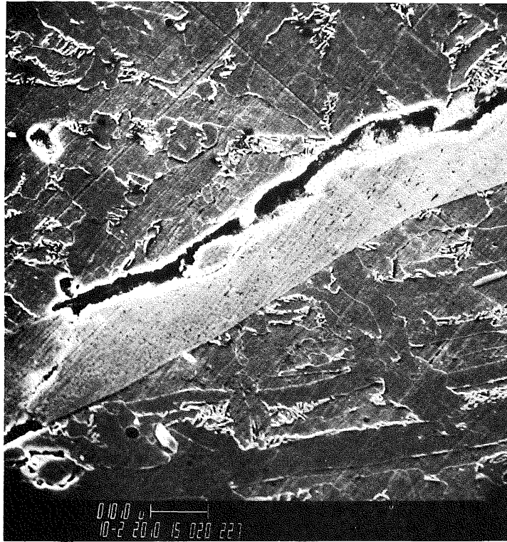
Fig. 51. SEM photograph of a crack filled with copper (Core F).
