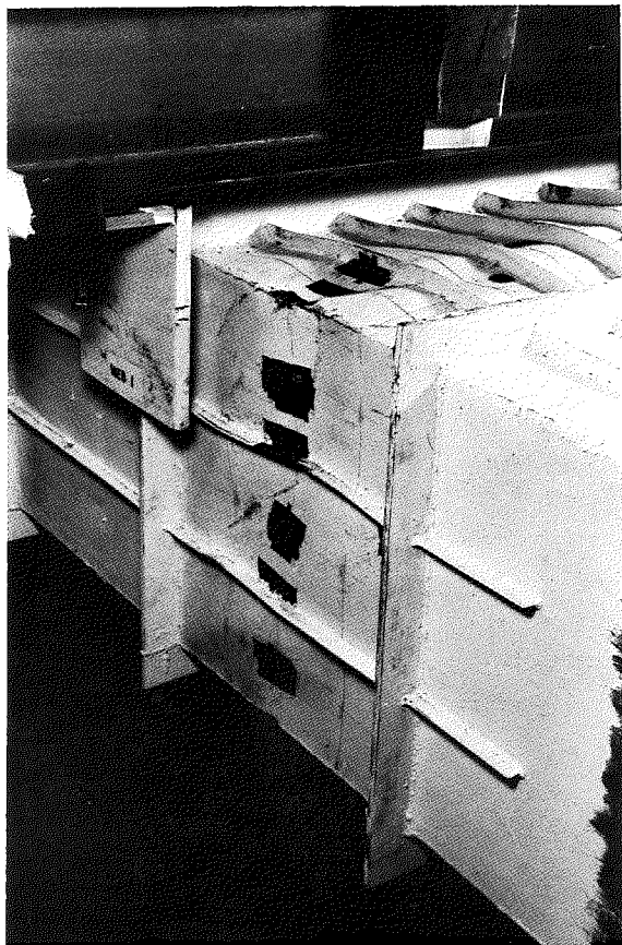
Fig. 37 Deformations of Compression Flange and Web 1 (Test 1)
