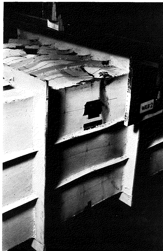
Fig. 38 Deformations of Compression Flange and Web 2 (Test 1)
