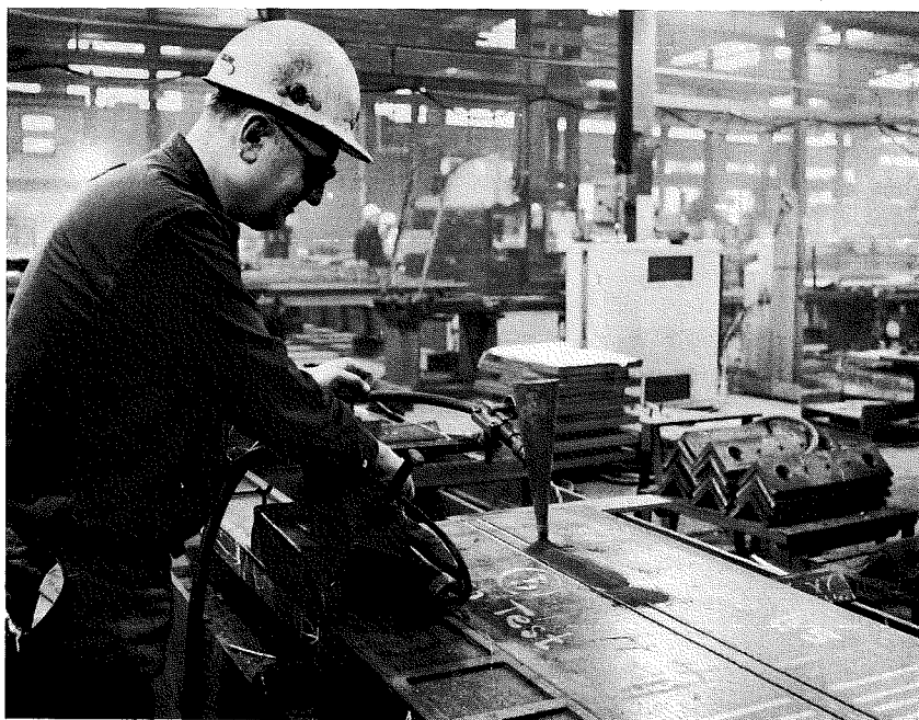
Fig. 17 Welding Process on a Plate 24" x 2".
