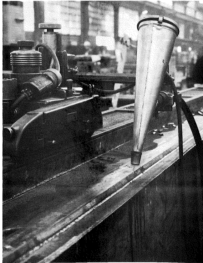
Fig. 18 Welding Process on the Box Shape 24 □ 774.
