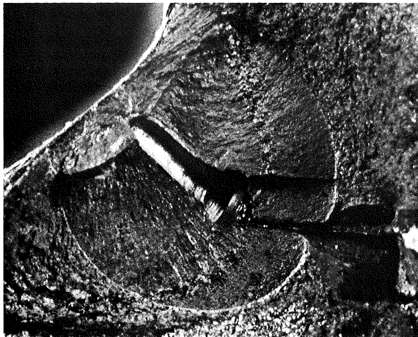
Fig. 24 Small crack with penetration to the fillet-weld surface ( \sim x11 )
