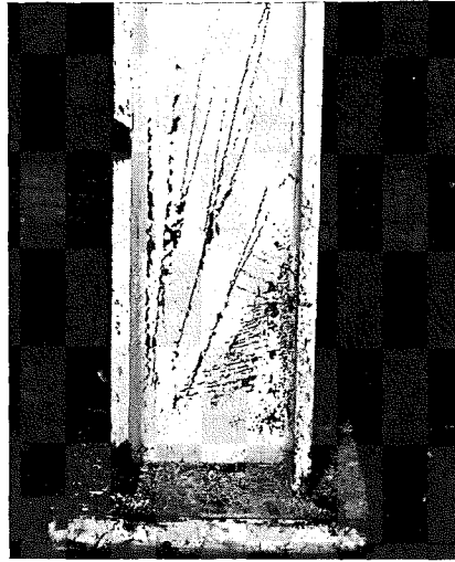
Fig. 21—Plastic region above base plate ( V = 216 kips)
