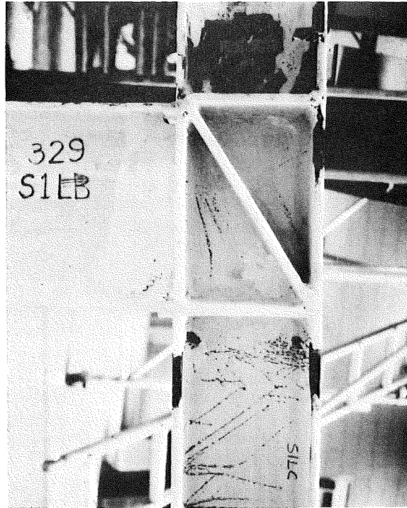
Fig. 28 Yielding in Column Below Lower Joint of Subassemblage S-1
