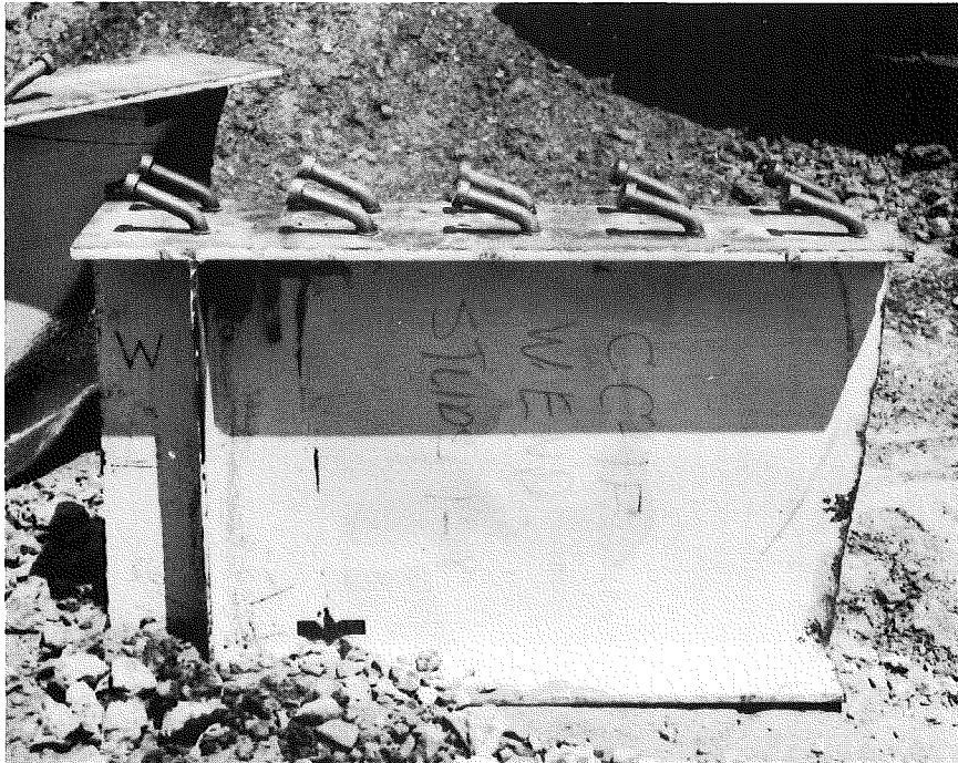
Fig. 13 Studs at the End of Beam CC-1F After Fatigue Testing
