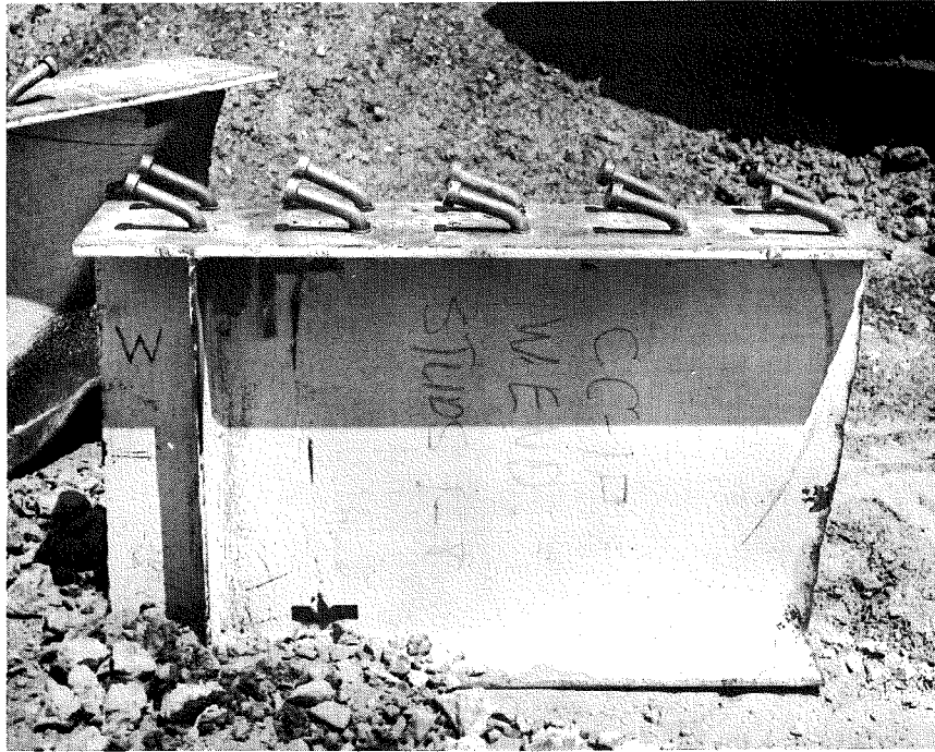
Fig. 23 Studs at End of Beam CC-1F after Fatigue Tests
